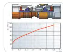
**EN.** Moulded internal profile: reduces pressure loss.
