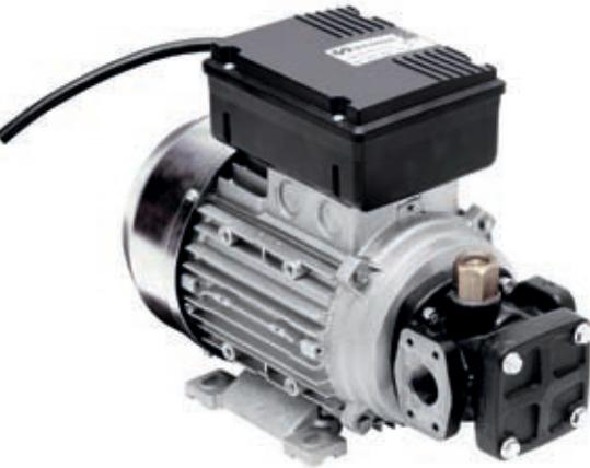
Internal gear electric pumps for lubricants. 230 V - 50 Hz (single-phase) or 380 V - 50 Hz (three-phase) motor, depending on model, IP-55 protection and on/off switch. Cast iron pump body, sintered steel gears and by-pass valve. Motor with mounting feet, the pump can be mounted horizontally on a flat surface or vertically on a wall.
